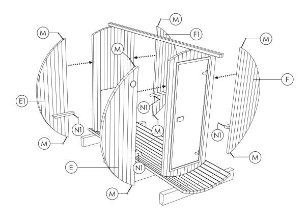
**STEP 6:** Continue placing left and right body staves (C, C1) tightly on both sides of the sauna using rubber mallet, and fixing body staves with screws 4.20x70. To finish the roof top joint, use roof finishing item (H). Item (H) has different thickness filling pieces. Combine them to fill the gap fully.
